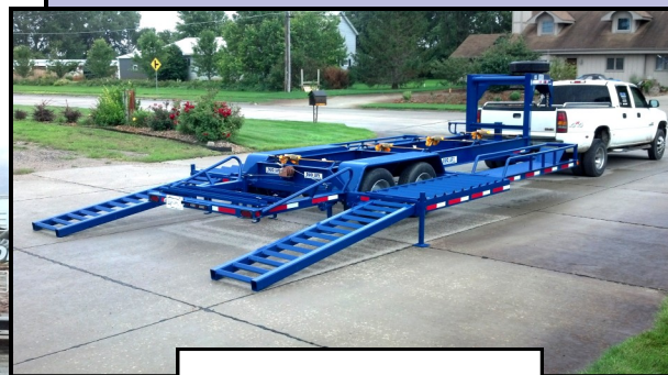
Guide Rails Keep the Rear Tires From Turning. Railing is Adjustable for Various Tire Sizes
