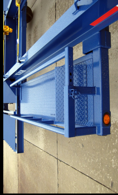
Adjustable Position Caster Wheel Platform Railings and Wheel Stops
